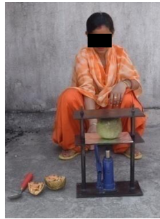
Fig. 10. Worker using shell cracker
