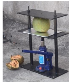
Fig. 8. Diagonal view of shell cracker
