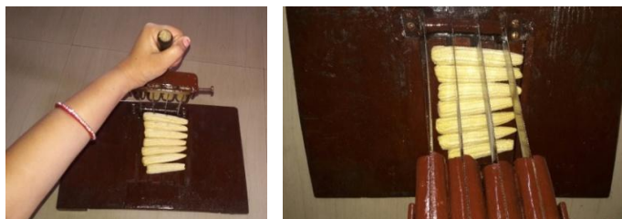
Fig. 5. Cutting multiple baby corns with veg-multi-slicer
