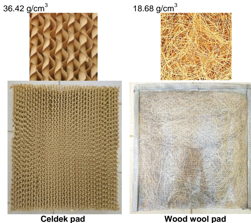
Fig. 1. Commercial Celdek pad (left) against locally made wood wool pad (right)
