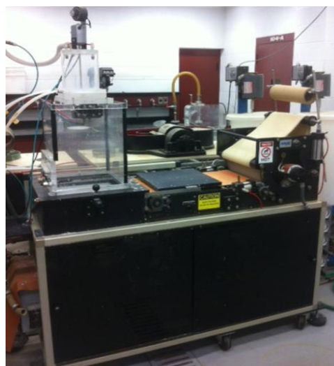
Fig. 3. MK Systems Inc. dynamic sheet former [25]
