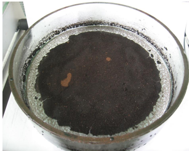
Figure 9. The appearance of the solidified oil layer after waves exposure during 1 hour.
