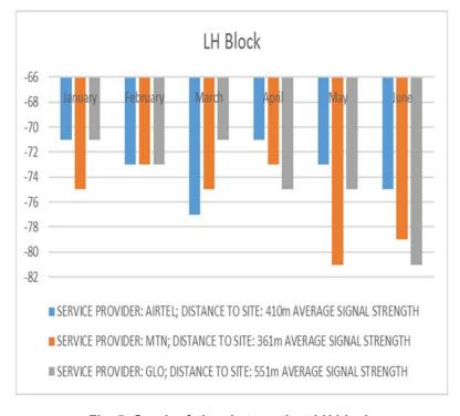
Fig. 5. Graph of signal strength at LH block
