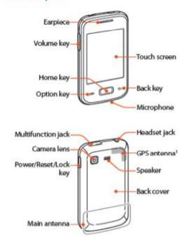
Fig. 1. Front view of the mobile device
