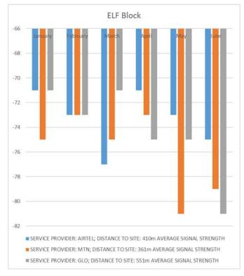
Fig. 7. Graph of signal strength at ELF block
