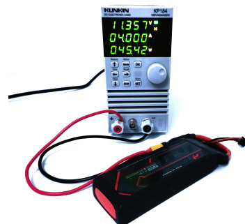
Figure 10. KP-184 programmable electronic load used to characterize the battery employed in the experimental platform.
