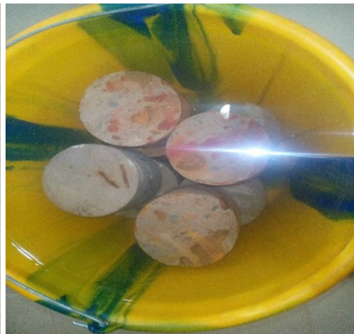
Plate 5. Curing of sample specimen for 24 hours
