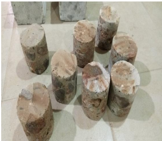
Plate 4: Cored Concrete mass samples
