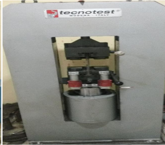
Plate 7. Tensile strength test of reinforcement steel sample
